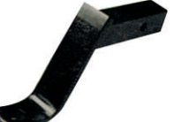
BM1005 Technical index: 6DROP 4-3/4RISE 9LENGTH max.tongue-5000bs classII Material:Hot roll steel Surface treatment:Coating
