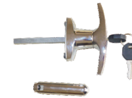
TP1428 Trailer Case Lock Zinc alloy,chromed Shafer:80×8mm Hander:100×30mm
