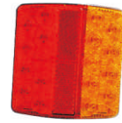
TL065 LED tail light Stop, rear position, rear direction indicator lamp W/o no plate lamp 100% waterproof Size: 106×100×46.5mm
