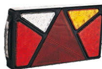
TL080 LED stop/rear position/rear direction Indicator lamp, reversing lamp Number plate light, triangle reflector, Fog lamp horizontal mount version Feature extra wide angle optics for Improved side visibility Size: 271×146×32mm
