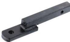
BM1001 Technical index: 1-1/4DROP 5/8RISE 6-1/2LENGTH max.tongue-3500bs classII Material:Hot roll steel Surface treatment:Coating
