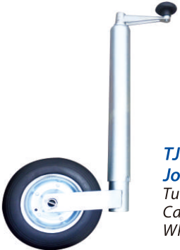
TJ1100 Jockey wheel Tube: \Phi 35 mm Capacity: 75kgs Wheel: 6inch
