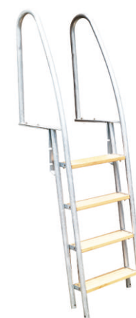
L8040 Dock Ladder Hot dip galvanized 4 Steps Total Length:2000mm Width:500mm Wood Steps
