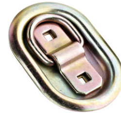
TP1043 Lashing Ring Hole:8×8mm, Cto c 45mm, Steel,zinc plated
