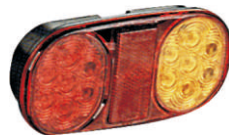
TL030 LED tail light Stop, rear position, rear direction indicator lamp Reversing lamp, w/o no plate lamp 100% waterproof Size: 162×80×26.5mm
