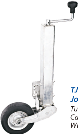
TJ1320 Jockey wheel Tube: \Phi 60 mm Capacity: 250kgs Wheel: 8inch
