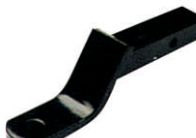
BM1004 Technical index: 4DROP 2-3/4RISE 9LENGTH max.tongue-6000bs classII Material:Hot roll steel Surface treatment:Coating
